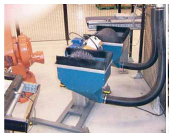
Robot deburring for telecom parts
