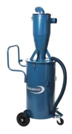
The DCF Mobile Cyclone has a high efficiency cyclone mounted on the top cover. Thanks to the small diameter of the cylinder in relation to its height and to the specially shaped inlet, this separator can separate even smaller and lighter materials such as asbestos fibres. The separated material then falls into the container which is fitted with a plastic bag for dust-free handling.
